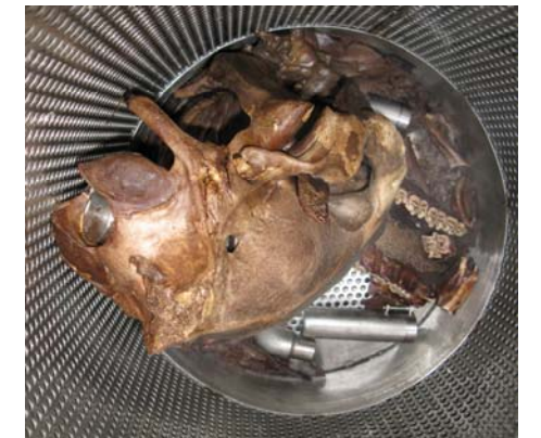
Horse skull with steel capsule after digestion cycle.
